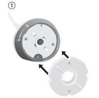
With light pressure turn the transmission disc ④ clockwise, until the resistance yields. The arrows on the transmissiondisc ④ and in the motor unit ③ must point to each other ∑ (See ill. ② – ③).
